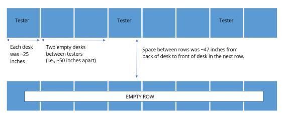
Second row of testers were staggered from first row (i.e., tester should not be in the same row).
